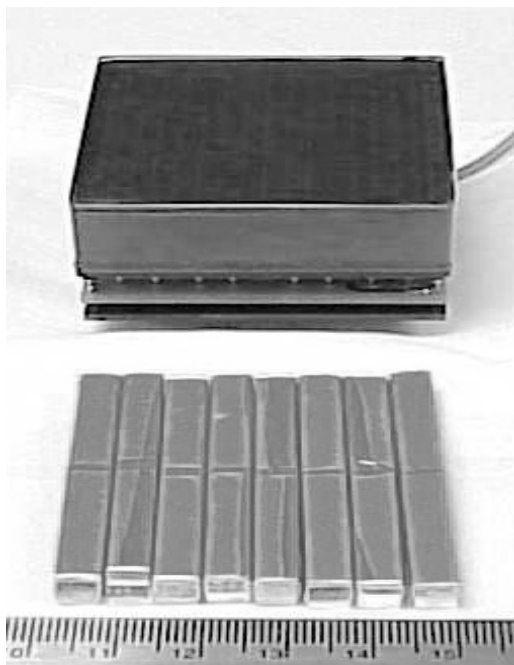
Figure 10: The Hamamatsu H8500 MAPMT (top), and several plastic scintillator elements (bottom).
