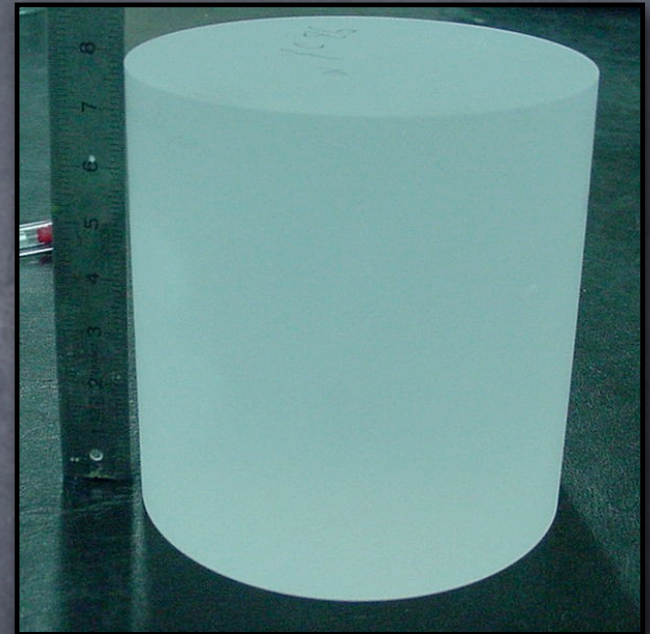
3" x 3" \text{LaCl}_3 (St. Gobain) \Delta E/E = 4.1\%
