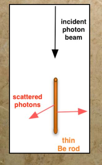
THE VALIDATION RESULTS PRESENTED HERE USE A SIMPLE SCATTERING GEOMETRY.
